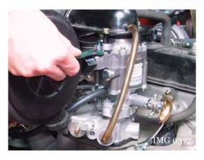
9. Set the power adjustment on the carburetor. With the wheels blocked parking brake on and foot on the brake pedal. In drive, depress accelerator to full throttle position. Set CO% to .80 CO%.
