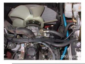
5. Route the fuel vapor hose and lock-off vacuum line to the carburetor along the path of the old hose. Secure in place with tie straps.
