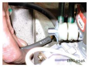
3. Disconnect the vacuum line from the regulator to governor plate, and plug the governor plate fitting with the supplied vacuum cap.
