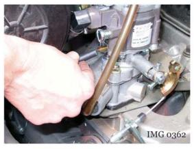
7. Connect the fuel lock vacuum hose to the large brass vacuum port on the carburetor.
