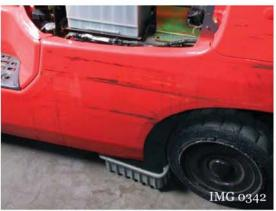
5. Place a drain pan under the lift to catch coolant when hoses are disconnected from the engine.
