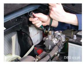
2. Disconnect the fuel line from regulator assembly.
