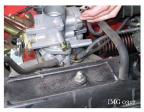
6. Disconnect the two vacuum hoses from the carburetor that lead to the governor plate.
