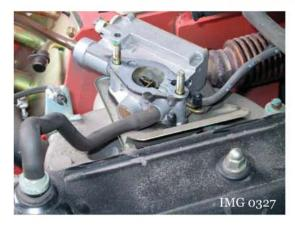
8. Disconnect the throttle cable. Remove the carburetor and gasket from the governor.
