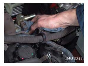
6. Disconnect coolant hoses from engine.
