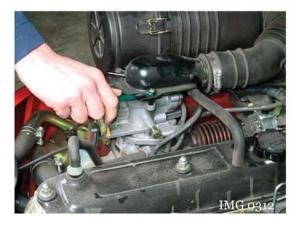
4. Remove the air plenum from the carburetor.
