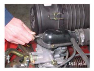
3. Remove the crankcase vent and governor air hose from the air plenum.
