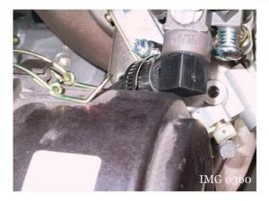
Connect the fuel vapor hose and clamp to the carburetor fitting and tighten.
