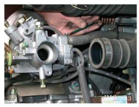
5. Disconnect the fuel vapor hose from the carburetor.
