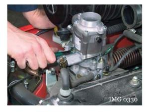
2. Install the IMPCO carburetor and fasteners. Tighten the nuts to 17 lb. ft. (23 N·m).
