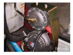
2. Connect the fuel line to the lock-off and torque to 20 lb. ft. (27 N·m).
