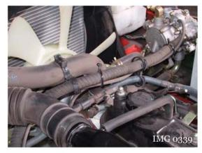
7. Remove vapor and vacuum hose from hold down straps.
