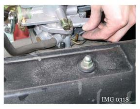
7. Cap the two vacuum ports from the where the lines were removed.
