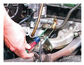
7. Set the engine idle speed at the carburetor to 800 RPM in neutral.
