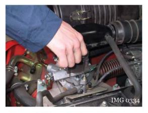
6. Tighten the plenum bolts to ll lb. ft. (14.9 N·m)
