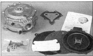
1.Under normal conditions, installation of a complete repair kit should be necessary only at the time of a major engine overhaul or when the regulator has been out of service for an extended period of time. Each kit includes the necessary gaskets, diaphragms, seals and some replacement screws.
