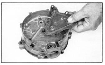
25. The new primary diaphragm assembly (13) is ready to be put into place.
