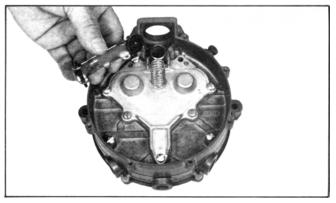
10. Remove the lever and seat assembly (5 & 6). **E Only:** Remove Spring (7).
