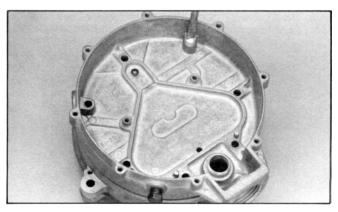
14. Remove the last two fillister screws (10).
