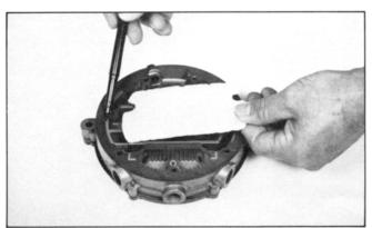
21. The pen indicates the recess cast in the body (19) to retain the sponge (17). Be sure to accurately install the sponge in the recess.
