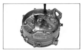
26. Install the primary diaphragm (13) over the locating pins and screw bosses, providing alignment for the assembly of the springs (12) and cover (11).
