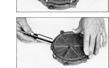
18. Tap the side of the cover (22) firmly with the handle of the screw driver to break the cover loose from the gasket (21).
