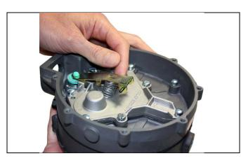
40. **Model E Only** (Skip for PE): Slip the spring (7) under the secondary lever (5) making sure it is retained by the two tabs at the sides and the single tab punched through the top of the lever.
