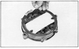
22. After the sponge (17) is in place, the primary seat (18) can be installed. Place the seat so the rubber side is down towards the jet.
