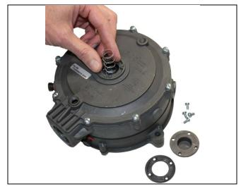
Model PE Only (Skip for E): Remove the spring retainer housing cover screws (27) and cover (28). Remove the housing gasket (29) and secondary spring (7).
