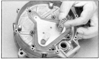
27. Place the two primary valve springs (12) on their locating perches extruded from the backup plate on the primary diaphragm (13).
