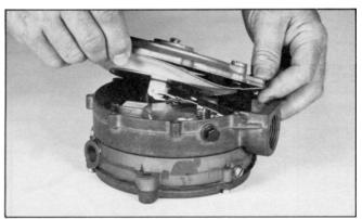
4.Remove the secondary diaphragm (4). This requires the assembly be moved about one inch away from the gas outlet to disengage the two prongs of the diaphragm link from the lever (5).
