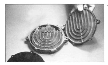
19. Deposits may accumulate from the use of hard water. This condition can be alleviated through the use of radiator additives or permanent antifreeze solutions. Remove any accumulation with a wire brush before assembly. Steel water inlet and outlet fittings may cause erosion from electrolysis. Use brass or plastic water fittings only.
