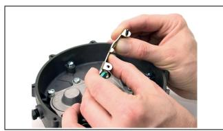
37. If necessary, remove the fulcrum pin (8) and lever (5) and bend slightly if required. Do not attempt to bend the lever when installed--unnecessary force on the lever may damage the secondary seat (6).
