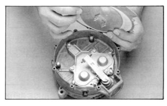
5.Diaphragm (4) and cover (3) removed showing secondary lever (5).
