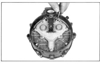
7. Extract the screw (10) in preparation for removal of the fulcrum pin (8).
