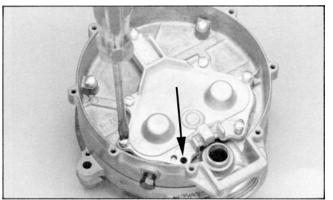
29. **Early Models:** Replace four of the five screws (10). DO NOT replace the one shown by the arrow. Torque to 35-45 in-lbs. (4.0-5.1 Nm). Torque the two inner screws (9) to 22-28 in-lbs. (2.5-3.2 Nm).
