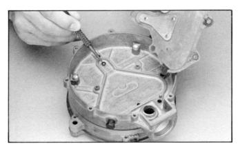
13. Remove the primary valve pin (14) as shown by the tip of the pen.
