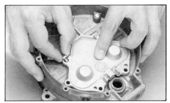
28. Press the primary cover (11) in place over the primary valve springs (12) and diaphragm assembly (13). Insert two screws (9) and finger tighten.
