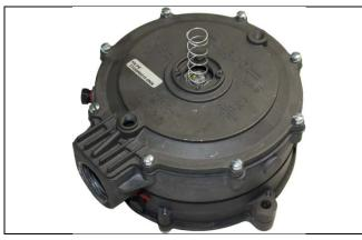
45. **PE Only** (Skip for E): Place the secondary spring (7) on the secondary diaphragm (4) perch.
