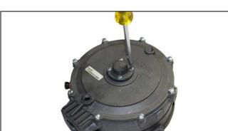
46. PE Only (Skip for E): Install the gasket (28) and spring housing (27). Align the spring retainer housing screw holes to the cover (26) and insert cover screws (23). Torque to 7-11 in-lbs.(0.8-1.2 Nm).
