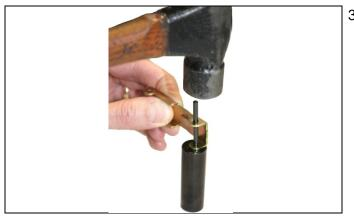
30. Slide the pin through the larger of the two hole openings of the lever (5) and place over a socket that will support the area of the lever around the hole. Using a hammer, knock in the pin (26) through the smaller hole until it is even on both sides.
