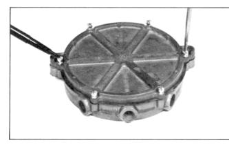
20. Reassemble the back cover (22) and gasket (21) to the heat exchanger body (19). Replace six screws (2). Match the mounting bosses in the cover with those on the heat exchanger. Tighten the two screws shown in the photo first, then upper and lower screws diagonally opposite to draw the cover down evenly. Torque to 25-35 in-lbs (2.8-4.0 Nm).
