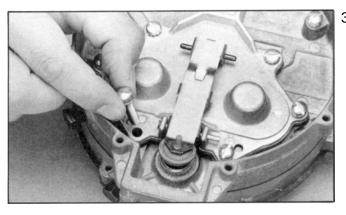
34. Replace the final screw (10) and finger tighten. Skip to Step 36.
