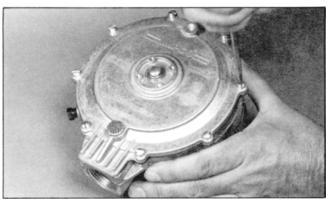
3.Remove the diaphragm cover (3) by taking out the eight screws (2) around the circumference of the top cover.
