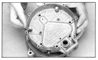
23. Reinstall the body (15) and body gasket (16). Mount the body gasket on the primary pin boss and two locating pins on the underside of the body. Use two screws (10) to locate the body on the heat exchanger body (19). Finger tighten the screws to hold the two parts in place.
