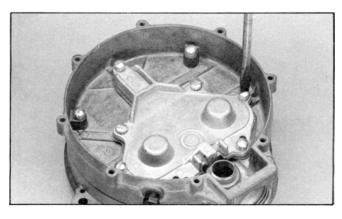
Remove the primary diaphragm cover (11). This requires removal of four fillister head screws (10) and two pan head screws (9).
