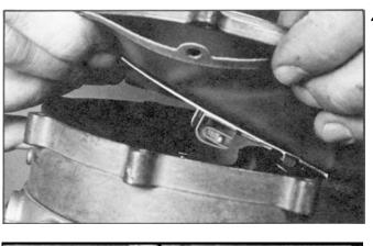
42. Photo shows the link and the link pin properly connected.
