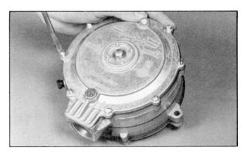
44. Replace the cover (3). Turn the eight screws (2) until all contact the cover. Then tighten in a crisscross pattern until are firmly seated. Torque to 25-35 in-lbs. (2.8-4.0 Nm).
