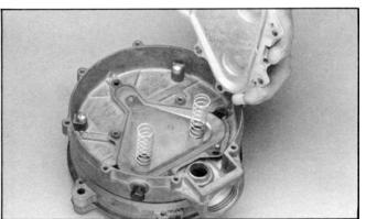
12. Remove springs (12) and the primary diaphragm assembly (13).
