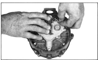
8. Slide out the fulcrum pin (8) and remove the pin.
