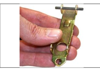
31. Inspect the tabs on the lever (5) to verify they are not bent and the pin (26) is centered.
