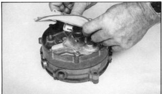
41. Replace the secondary diaphragm (4) engaging the slotted link to lever pin shown.
