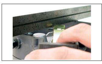
36. Lightly pull the lever (5) up against the secondary seat for measuring. Use a straight edge or the IMPCO G2-2 gauge to check the lever height. The secondary lever link pin should be approximately 1/32" (0.8mm) below the level of the body casting. If the lever height is incorrect, continue to Step 37. Once the lever height is correct, skip to Step 38.
