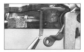
13 Install spring as shown through spring perch hole in W1-21-2 washer and through hole shown in lever to pull lever upward and out of operation. Wire may be used to hold lever up if spring is missing.
