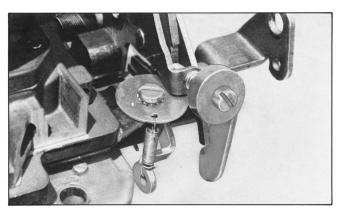
14 Illustration shows completed idle stop screw assembly.
