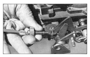
Using new S1-51 idle screw (10-32 x 1-1/4"), place the W1-40 washer next to the screw head, then install idle stop spring (S2-15) on screw and thread assembly through the fast idle lever. Weight of the washer holds fast-idle lever down against the W1-21-2 washer below, and maintains a permanent position for the idle adjustment screw.
