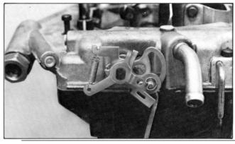
12 On the fuel inlet side of the gasoline bowl, locate and remove the small spring for use in next step.
