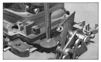
Fasten washer in place as illustrated with 3/32" spring perch hole in line with the lever directly below.
