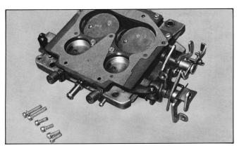
7 A3-64 adapter attached to throttle body, ready to fasten to mixer assembly.
