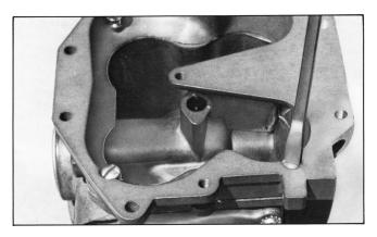
6 Fasten A3-37-2 adapter to CA425 mixer prior to assembly to the A3-64 adapter which has been mounted on the throttle body.
