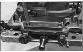
8 Use remaining two S1-65 screws (10-32 x 1") and W1-5 lockwashers as shown to fasten both adapters to the throttle body. Use four S1-71 (10-24 x 1/2") screws in four remaining holes, located at opposite side of adapter, to fasten the A3-37-2 adapter to the A3-64 adapter. Assembly of mixer to throttle body is now completed.
