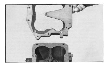
AA3-37-2 adapter assembly and CA425 mixer (bottom) includes four S1-19 (12-24 x 5/8") screws and G1-74 gasket. Photo shows screws in adapter and gasket in position on mixer
