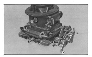
With completed carburetor in upright position as shown, front and rear flies should now be mechanically linked with no "monkey motion" in the operation. A small adjustment (bend) upward on the horizontal tab (arrow), may be necessary to align floating lever on the rear throttle shaft, so that the linkage is engaged each time the throttle is opened.
