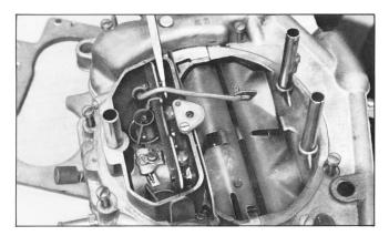
1 Remove eight screws around diameter of Carter gasoline bowl cover.
