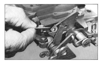
9 The idle adjustment makes use of the cold-start fast-idle lever shown at tip of washer. First, remove original fast-idle screw and spring as shown. In order to position the fast-idle lever so it will not move, the W1-21-2 washer (1" diameter with 3/32" offset hole) is fastened in the tapped 10-32 hole shown below the screw.
